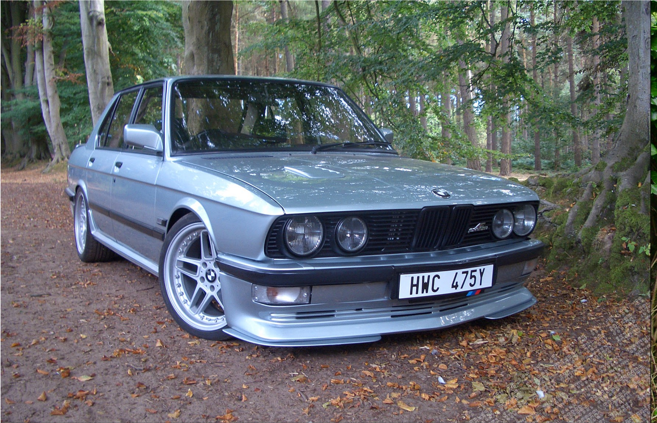
Oldschooldaddy's 1982 e28 528i in Sapphire blue, Leather interior, Zender body kit, Zender centre exit exhaust and front splitters, m30 3.5 Turbo charged engine, Hand built suspension > e34 540i big brake upgrade, Dog-leg box, LSD, Custom boot spoiler, Single wiper windscreen conversion, AC Schnitzer styling inc. 18" wheels, AC badging, AC steering wheel and pedals >>>
