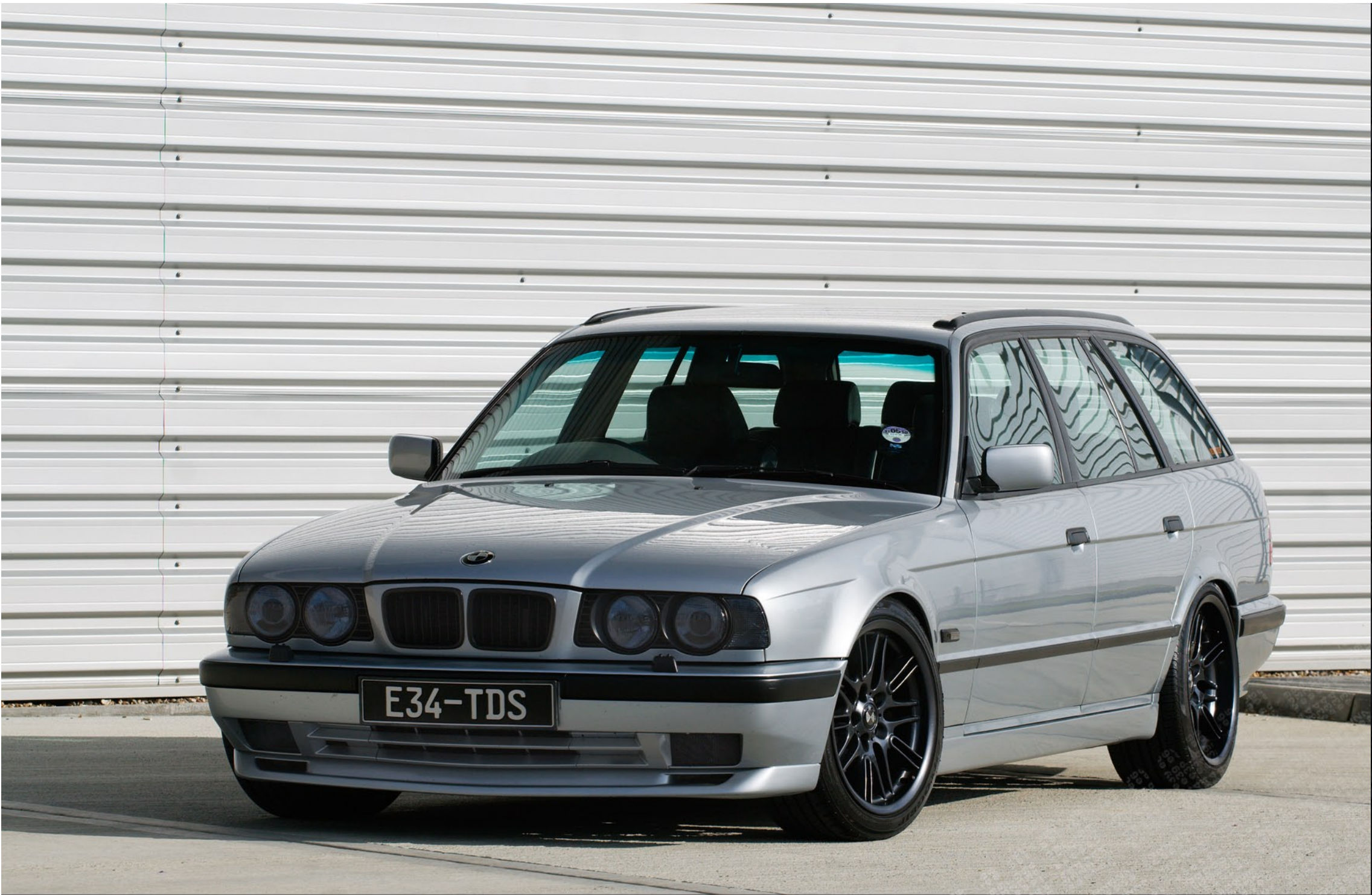
Tommy's e34 525 tds Touring with 18" E39 M5 Alloys 8.5x18 front 9.5x18 rear, Lowered suspension, M5 Front/rear bumper, M5 door kick-panel trim, De chromed front grill, Smoked Front > Light/indicators, All Red Rear Lights, 55w 6000k Hid, Carbon Badges all round, Custom exhaust system, Dark Grey Leather interior with front Elec memory Recaro's, Piano Black trim >>>>
